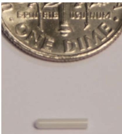
**Figure 2.** Ferrule used for implantation of optical fiber into the brain.
